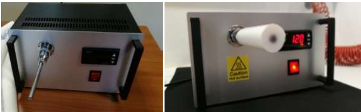
Figure 1. Photos of a measuring device for checking copper tube insulation materials for resistance to high temperatures
