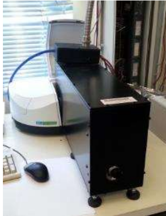
Figure 3. Heated transmission line and measuring cell, for spectral analysis of gases with FTIR
